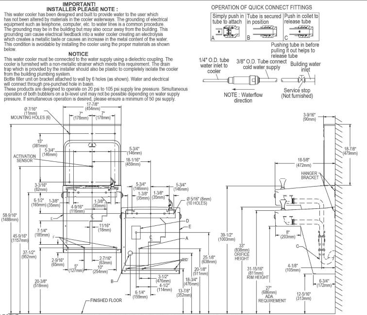
LEGEND: REDUCE HEIGHT BY 3 INCHES FOR INSTALLATION OF CHILDRENS ADA COOLER A = Recommended Water Supply location. Shut-off Valve (not furnished) to accept 3/8" O.D. unplated copper tube. Up to 3" (76mm) maximum out from wall. B = Recommended Waste Outlet location. To accommodate 1-1/2" nominal drain. Drain stub 2" (51mm) out from wall.
